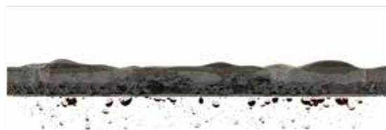
Conventional Flat Screen Solids Impede Fluid Flow
