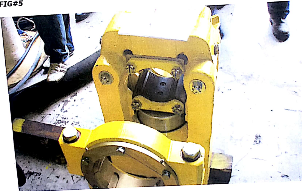
The pipe clamp was function tested and operated correctly in both directions.
